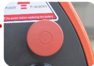
Emergency Power-off Switch
