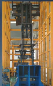
Fatigue test of lifting system
