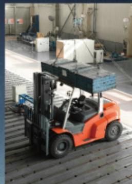
Impact test of overhead guard
