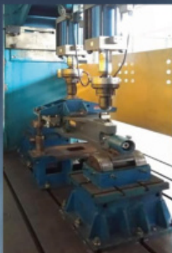
Fatigue test of steering axle
