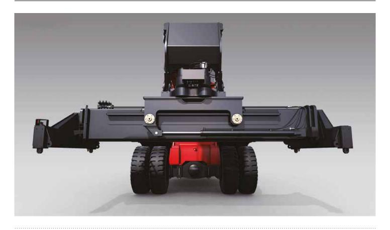
• 817 type spreader from world famous spreader manufacturer———Sweden ELME is assembled on the truck. The spreader is designed for reach stacker. The spreader is made by high—quality steel and it has single—cylinder type structure, high strength and good view.
