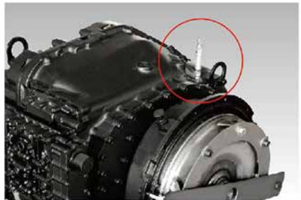
▪ Transmission box dust proof vent
