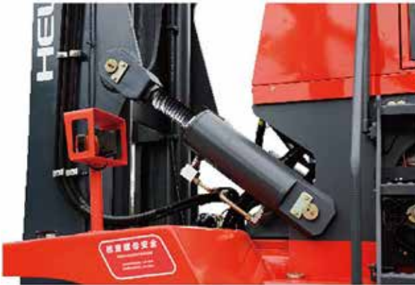
Oil cylinder protection sleeve(optional): it is used to protect cylinder damaged from foreign matters
