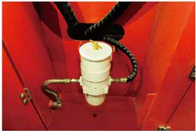
Steel wire winded hoses are used and safety level is improved greatly.
