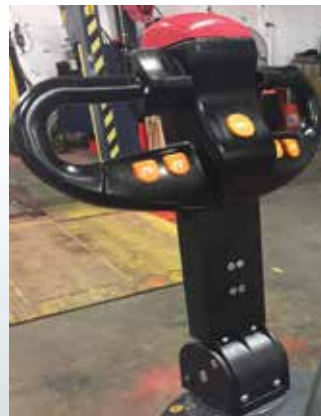
Ergonomic control handle with fingertip buttons
