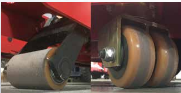
Polyurethane load and caster wheels have sealed bearings and are easy to service
